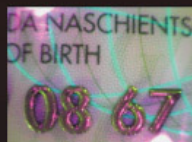
Guilloche and date of birth under UV light - UV fibers - Intaglio print under IR
