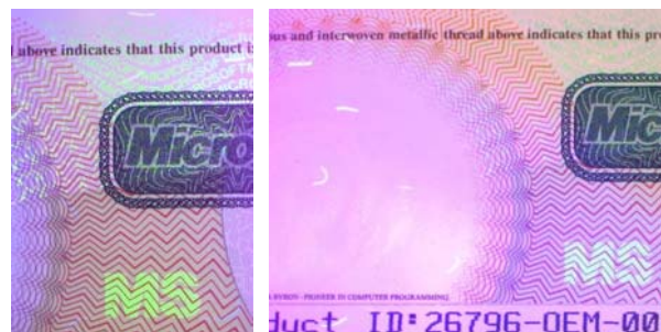
Figure 6 e 7 – MicroSoft® authenticity certificate with UV print and fibers.
